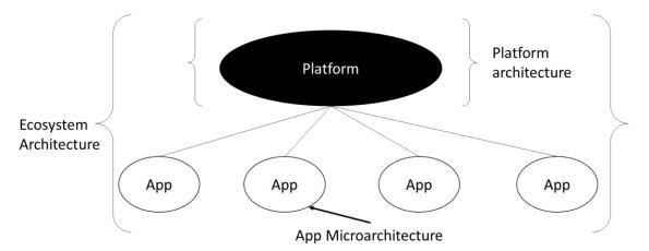
Figure 20. Ecosystem architecture as comprised of platform architecture and app microarchitecture (Tiwana 2014, p. 85).
