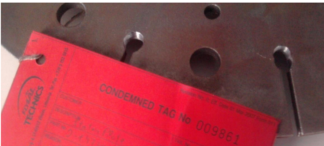
Figure 18-5. Brake stator plate. Cracks from holes
