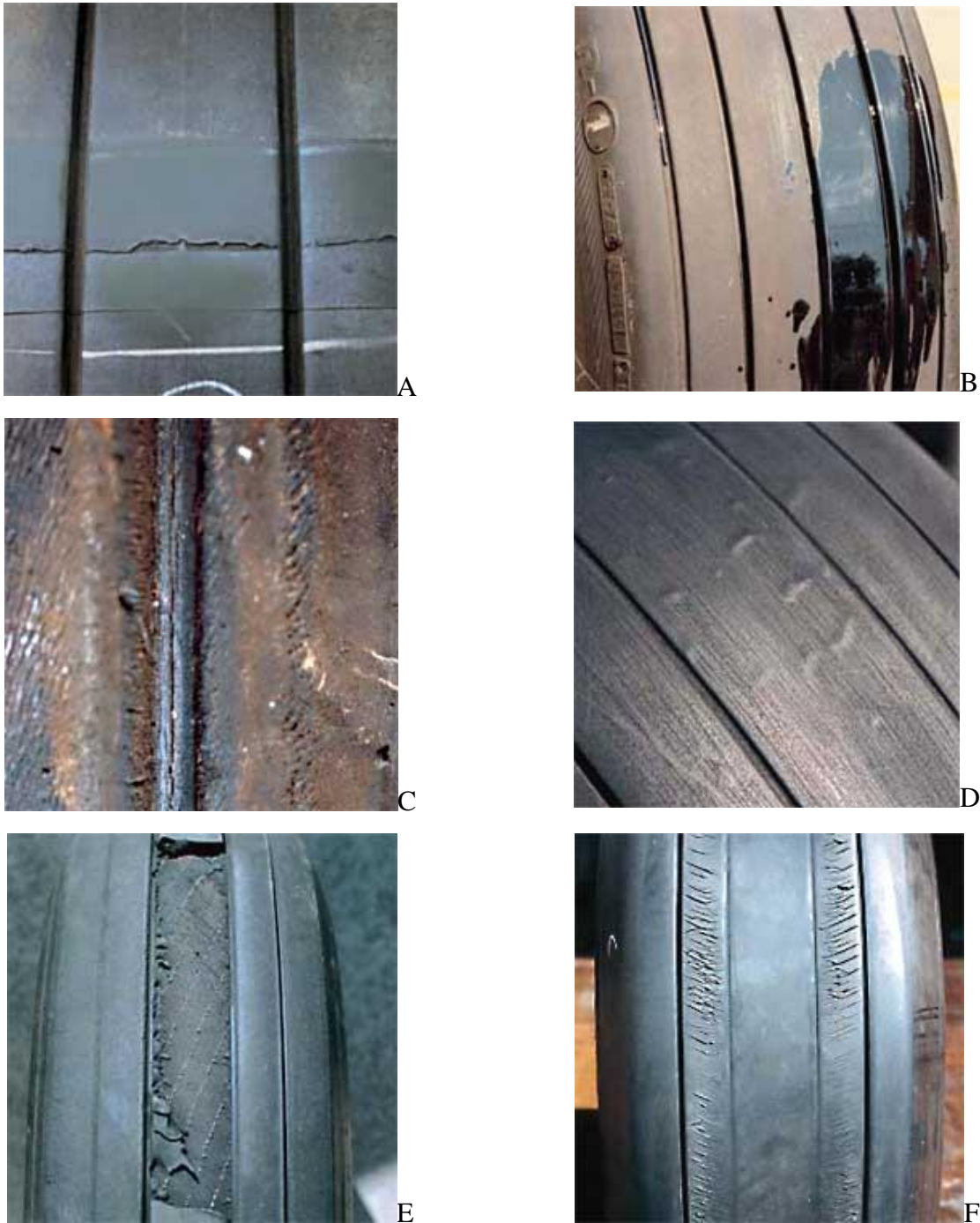
Figure 18-1. Aircraft tyres defects
