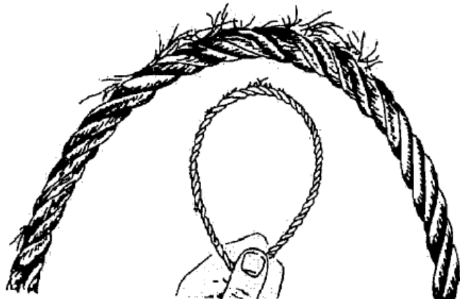
Figure 13-5. Inspection for broken wires
