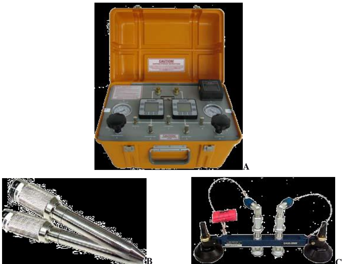
Figure 4-1. Pitot-static leak tester (A), Pitot adapters (B) and Static port adapter (C)
