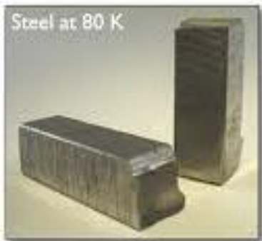
Figure 1-3. Brittle (left) and ductile (right) metal fracture
