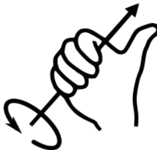
Figure 5-2. The right-hand rule of screw threads
