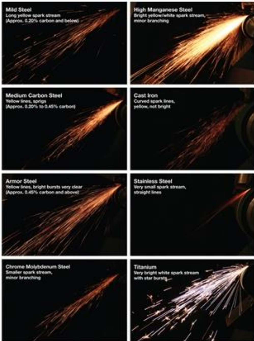
Figure 1-2. Spark testing
